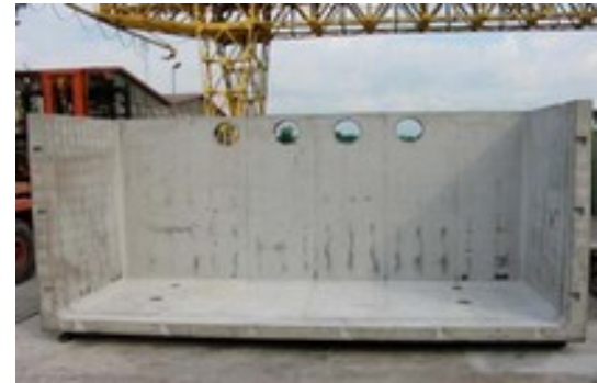
Examples of concrete bioreactor type vessels
